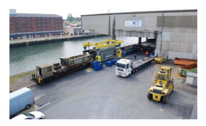
Unloading a transformer with 180 tons out of a railway wagon
