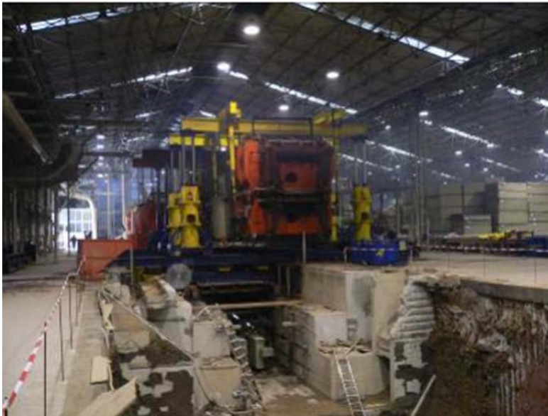
Particle board press in Sebes- Rumania Lifting out of the pit and moving sideways of 14 segments at the same time, weight 480tons. Use of 8 synchronic lifts
